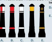
bands.\* D. 1 x 125mm Yellow retroreflective band.# 1 x 20mm and/or 1 x 38mm
