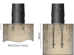
Adjustable depth concrete-in anchors
