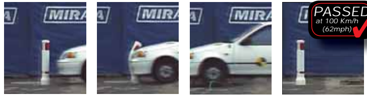
The first Glasdon socketed bollard proven passively safe to Performance Standard NE4/100.
