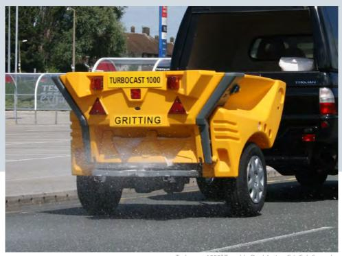
Turbocast 1000™ Towable Dual Action Grit/Salt Spreader
