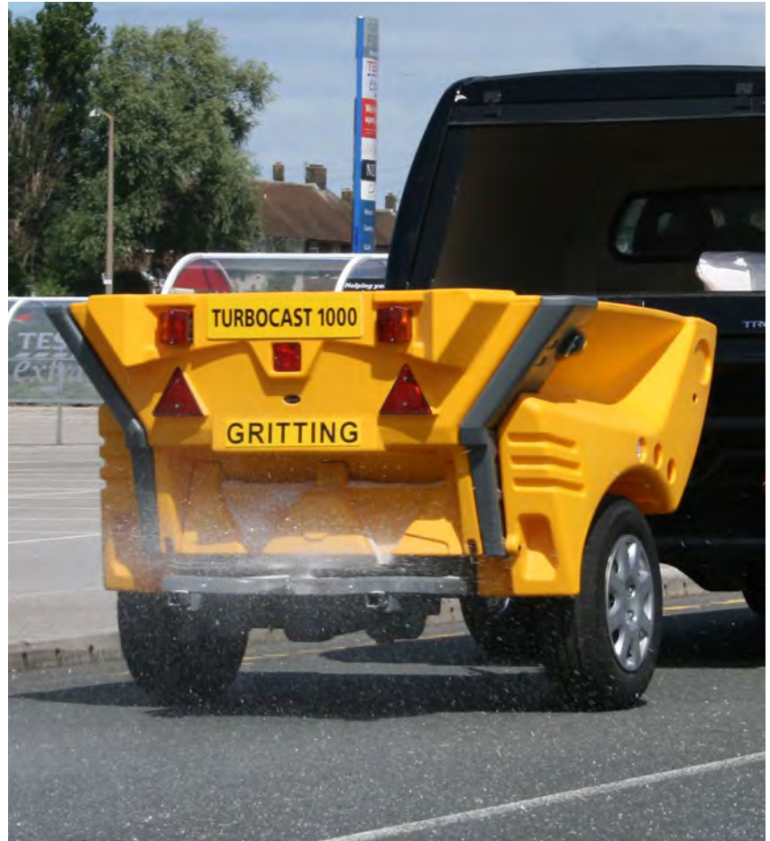
Turbocast 1000™ Towable Dual Action Grit/Salt Spreader
