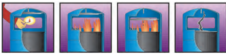
STAGE 1 A burning match is carelessly discarded into a litter bin. STAGE 2 The fire takes hold. STAGE 3 In under a minute, the fire extinguishing plate drops onto the liner. STAGE 4 The fire is contained.
