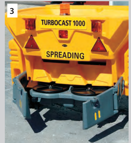
3 Repeat the procedure for the second side deflector to complete the conversion.
