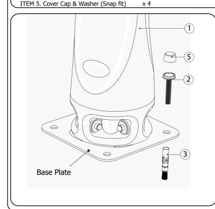
• Position the Bollard (Item 1) on to the intended site. Ensure reflectors are positioned in the correct orientation- red reflector faces oncoming traffic on the near-side, white reflector faces oncoming traffic on the off-side.
