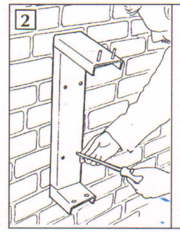
Drill the wall using masonry drill bit No 14 (9/32") and plug with the wall plugs provided. Screw the bracket to the wall using 4 off 21/2" long No 12 screws provided.
