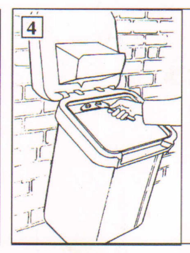
Open the lid and expose the protruding bolt studs at the back of the bin. Place the washer plate over the protruding bolt studs and secure the Retriever Bin with the nuts provided.
