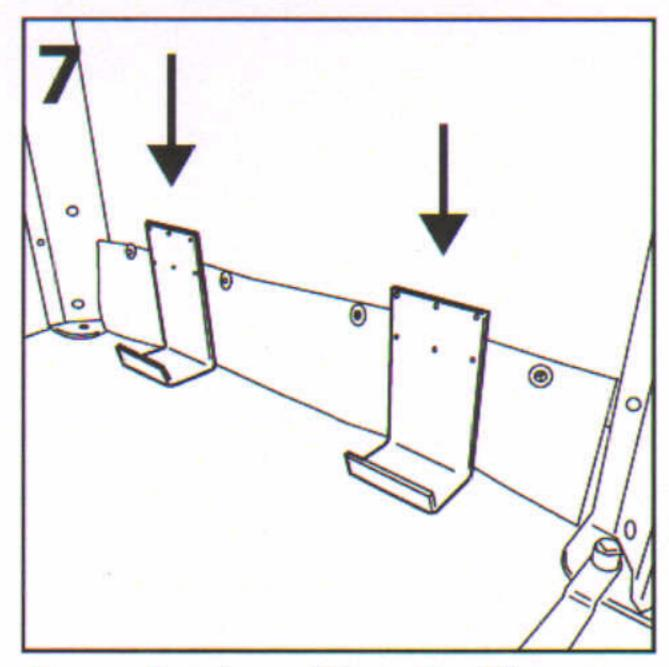
Open the door. Place 2 off bottom brackets (F) in between the fixings on the base skirting so that they are resting on the ground.
