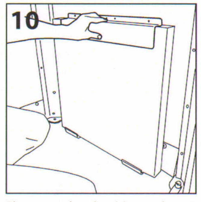
Place a top bracket (J) over the top of the paving slab and position centrally to the slab.
