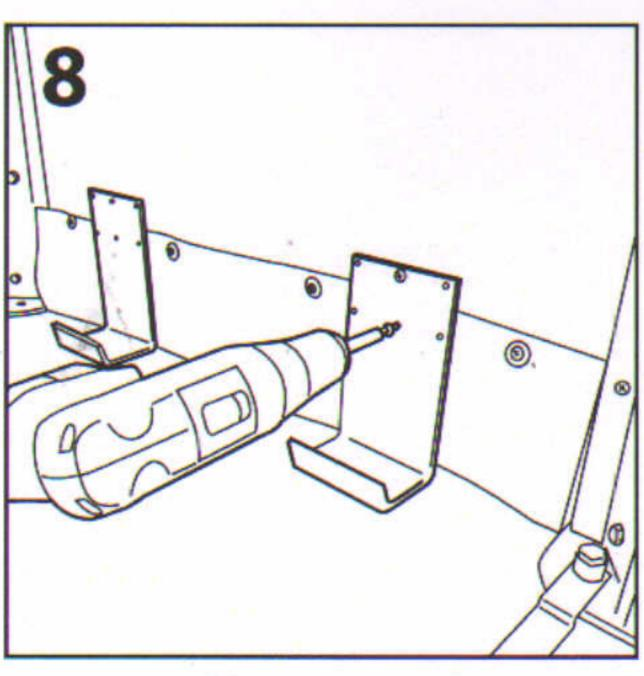
the pre-drilled holes in the brackets into the board.
