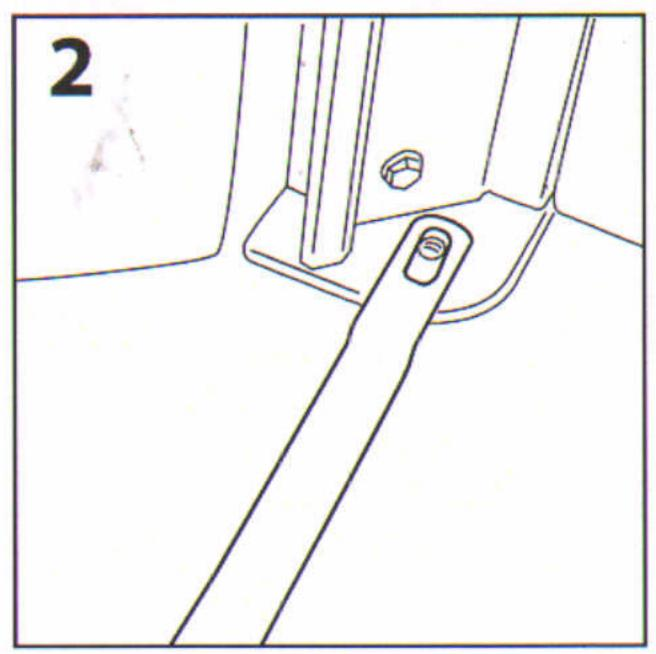
Lift up both of the front extrusions Place the ballast strap (B) between the front two extrusions so that the hole in each end is positioned over the Tee nut. Ensure that the ballast strap is resting on the ground.
