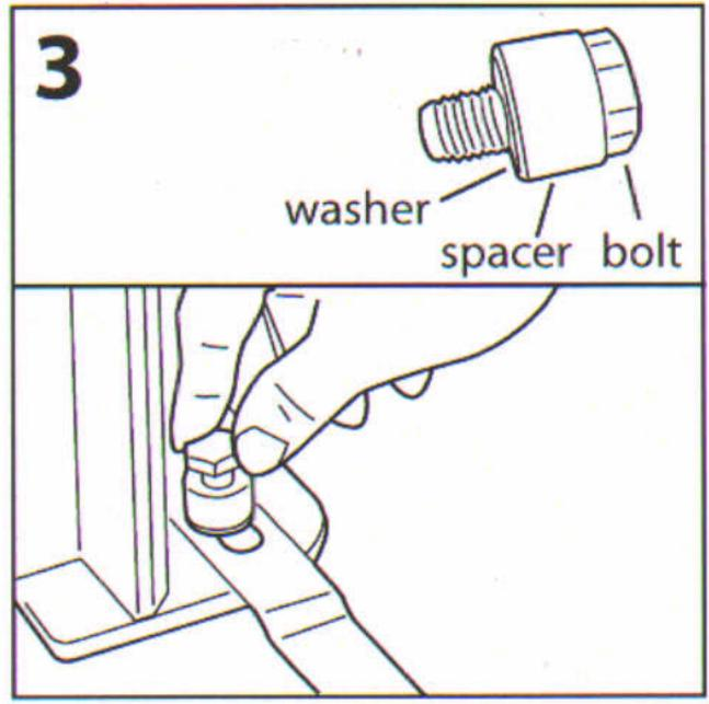
Using an M10mm bolt (C), 12mm spacer (D) and an M10mm washer (E) fix the ballast strap by hand at both ends using the fixings.
