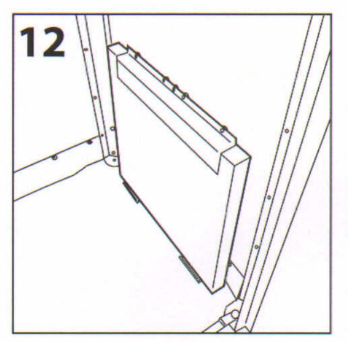
Repeat Figs 7 - 11 using the remaining two paving slabs so that both sides of the housing and the rear have a fixed ballast weight.
