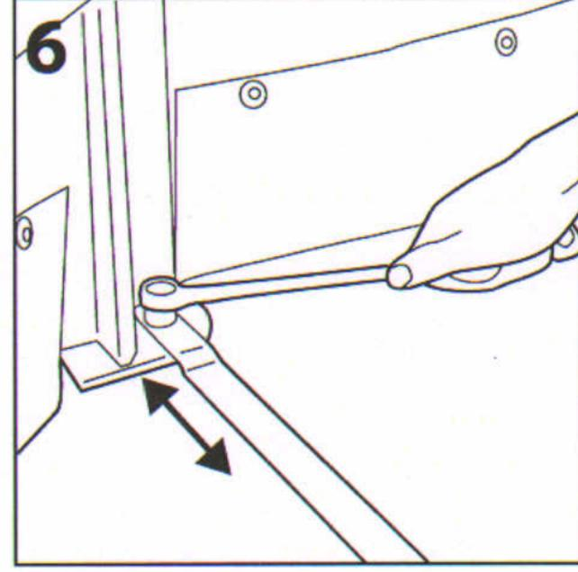
If the gap is uneven, unscrew the ballast strap fixings and adjust the position of the door receiver extrusion. When the gap is even secure the ballast strap fixings in place as per Fig 4.
