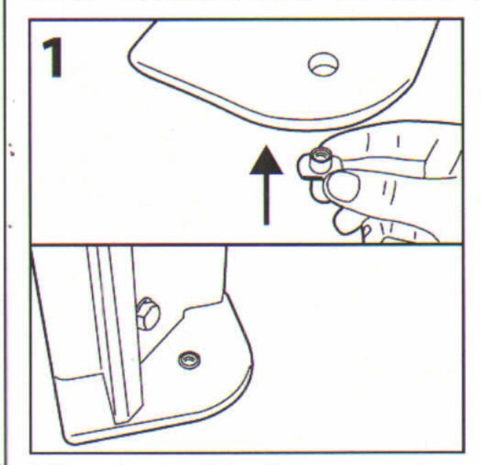
by tilting the housing backwards. Place a Tee nut (A) into the hole within each spigot plate from underneath so that the thread appears within the hole. (Will require 2 or more people).
