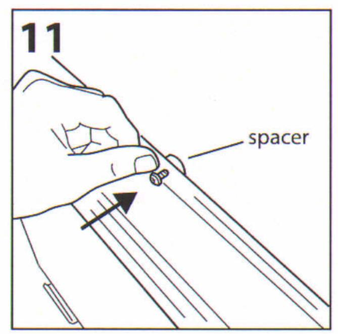
Using 5 off screws (G) and spacers (K), place the spacers in between the bracket and the panel and fix through the pre-drilled holes into the board.
