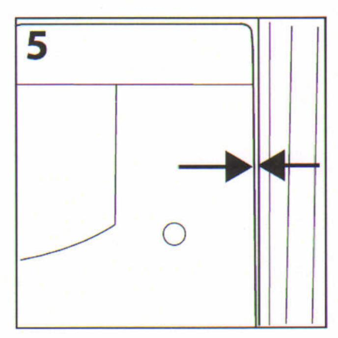
Close the door and ensure that there is an even gap running between the door and the receiving extrusion.
