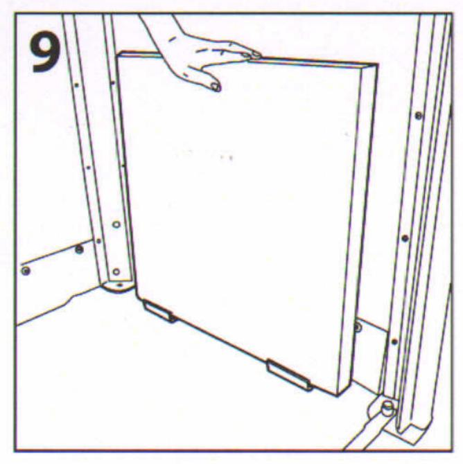
Using 12 off screws (G), fix through Using the correct size concrete slab (H or I, see table on page 1), lift the slab onto the bottom brackets so that it is positioned centrally (may require 2 people).
