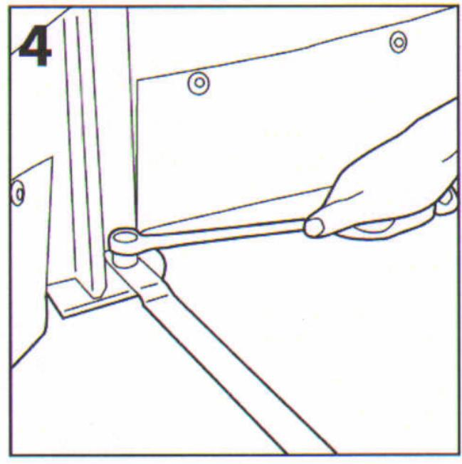
Using a 17mm spanner, secure the ballast strap in position at both ends.
