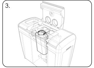
Empty the liquid reservoir by lifting it from the unit by the carry handle. Pour away the contents.
