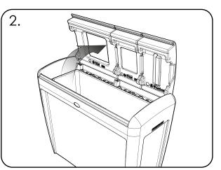
Open the lid to 90 degrees by pushing past the bump feature until the lid rests in an upright position. To close the lid pull the front down firmly to override the bump feature.
