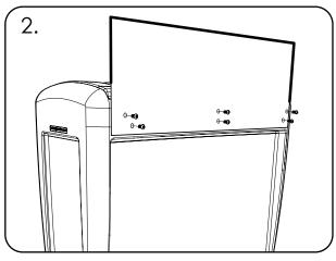
Position the sign carrier (item 1) and align the six fixing holes on the rear of the unit.
