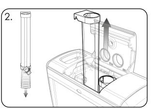
Lift the stacker off the support fixings. Use the quick release mechanism to release the cups. Place the stacker back onto the support fixings.
