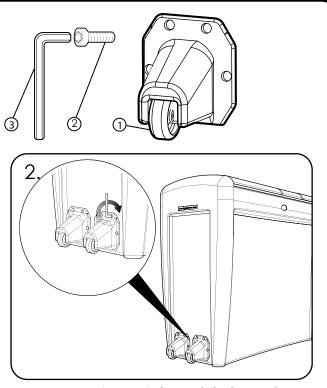
Insert screws (Item 2) through holes and tighten using Allen Key (Item 3).
