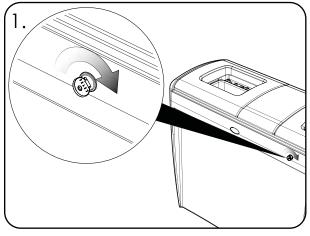
To unlock, twist key to 45 degrees clockwise until the barrel retracts.
