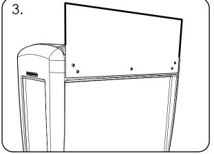
Fit the washers (Item 2) onto screws (Item 3) and fix through the holes in the backboard using Allen key (Item 4) to tighten.
