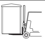
Short forks will damage the floor (if fitted) or will not support a Housing without a floor.
