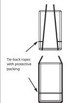
Slings must be seated at each end of the Housing and positioned approx. 250mm fro the corner for maximum stability.
