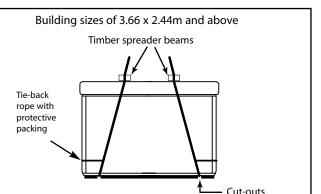
Position the slings in the cut-outs provided in the timber base plinth.
