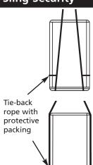
Slings must be seated at each end of the Building and positioned approx. 250mm from the corners for maximum stability.
