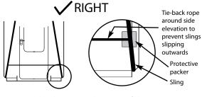
Position the slings at each corner of the Building on the underside of the panel base perimeter radius.
