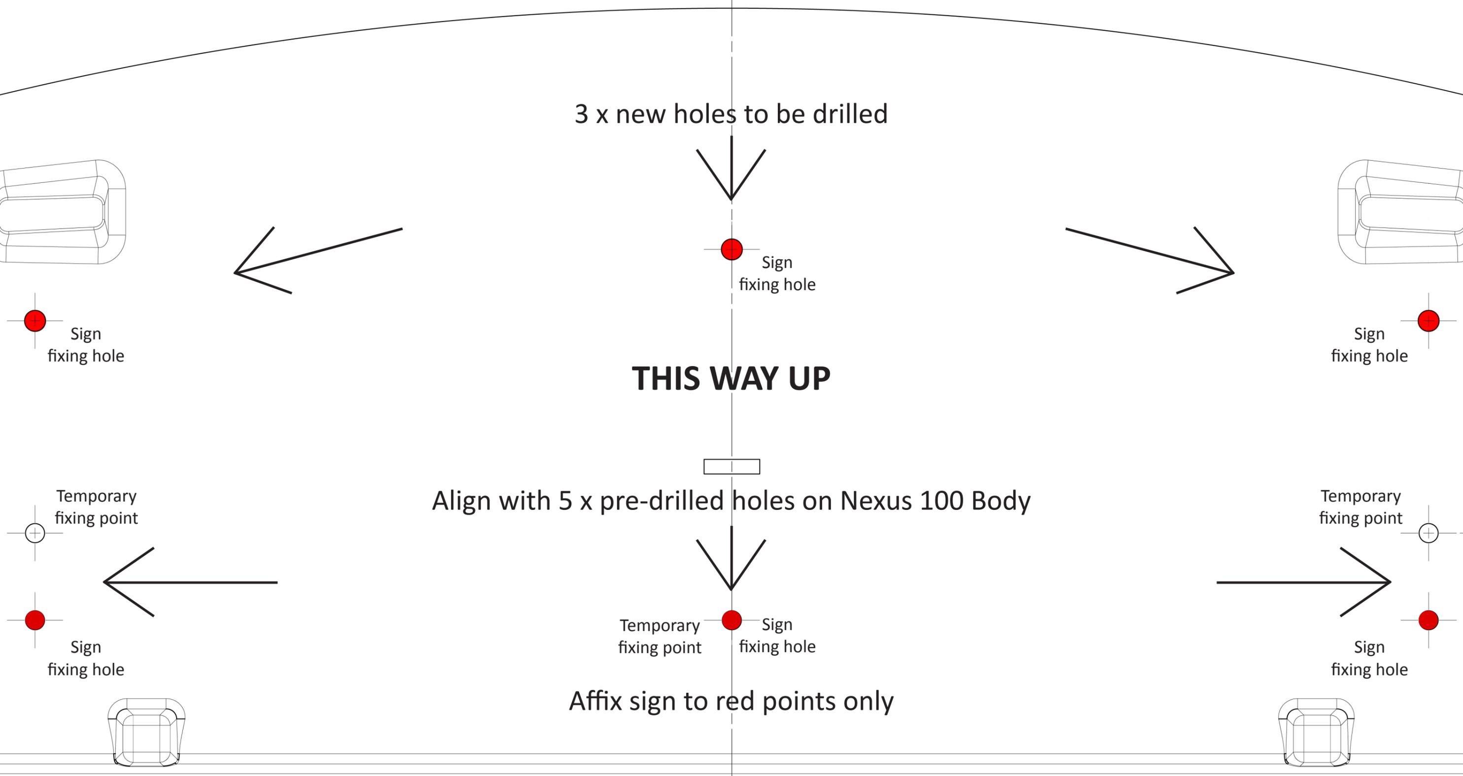
3 x new holes to be drilled
