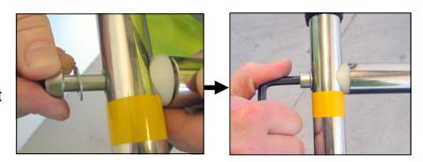
5) Holding the free end of the cross bar and a saddle washer together, push the handle bar towards the outside wall and position the cross bar onto it. When in position secure the cross bar using an M8 x 50mm screw and washer as in step 4.
