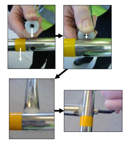
6) Place a cover cap ring onto a M6 x 40mm socket button screw and attach into either of the two inserts on the side of the Skipper using the 4mm allen key.
